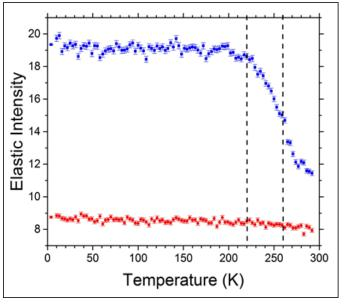
Quasi-elastic neutron scattering (QENS) scans of dry and hydrated deuterated cellulose. Data collected at 0.9 Å<sup>-1</sup> are shown. The scans at other Q values showed a similar trend. The data curves with blue squares and red circles represent the hydrated and dry samples, respectively. The dashed lines denote inflection points in the curves at 220 and 260 K in the hydrated cellulose sample.
