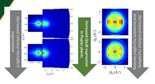
Graphic shows changes in Poplar cell wall structure with increased expression of 3-dehydroshikimate dehydratase (QsuB). Left panel shows 2D Small angle neutron scattering (SANS) detector images of wild-type (top) and QsuB1 mutant bottom. Right panel shows the corresponding wide angle X-ray scattering (WAXS) images.
